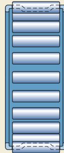
Sheet steel cage of the radial bearing
